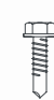
Tornillo Autotaladrante de cabeza hexagonal 4.8x19 Self-drilling screw with hex head 4.8x19 Vis autoperceuse à tête hexagonale 4.8x19 Саморез с шестигранной головкой 4.8x19
